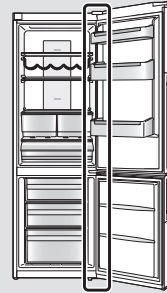
Potential pinch point
